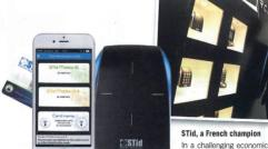
These social changes have led STid to draw on its experience to develop the STid Mobile ID solution. STid Mobile ID has been developed with RFID, NFC and Bluetooth Smart technologies, transferring an access badge to a smartphone, to work alongside or replace traditional badge technologies.
